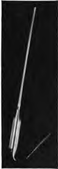
Fig. 96.—Special blood pipette (Miller).
